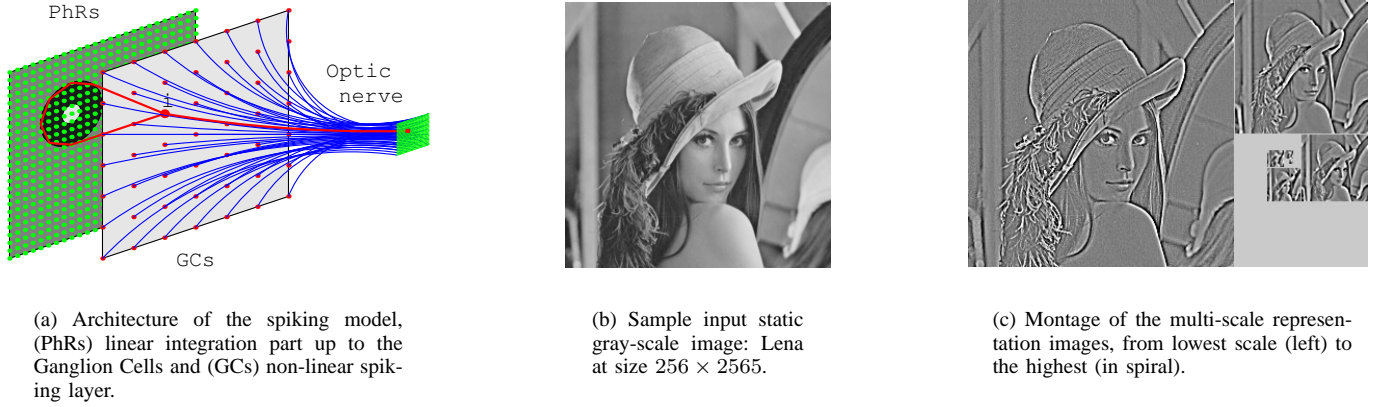
Fig. 1. Architecture of the model retina. 1(a) The model retina consist of two layers : an input layer corresponding to the photo-receptors (PhRs) which transmits the information analogically and linearly to the output layer corresponding to the ganglion cells (GCs). A sample GC neuron i is highlighted in red, and we showed its center-ON receptive field soma and axon. These ganglion cells produce spikes along their axons (forming the optic nerve). 1(b) The input of the model consist of static gray-scale images sampled over a rectangular grid (a white pixel corresponding to high luminance) which elicit the activity of the photo-receptors. 1(c) The model retina induces the activity of the ganglion cells which represents either positive (represented as white pixels) or negative (black) contrasts at different scales. We represented here for clarity the lowest scale (therefore at the highest frequency) with the left-most image and in a spiral the progressively down-sampled images of contrast values for progressively higher scales ( i.e. lower frequencies). Note that most values are gray, i.e. of low activity : the distribution of coefficients is kurtotic .
