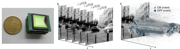
Figure 1: A miniature event-based ATIS sensor (Left) which, compared to classical frame-based representations (Middle), outputs an event-based representation of the scene (Right).
